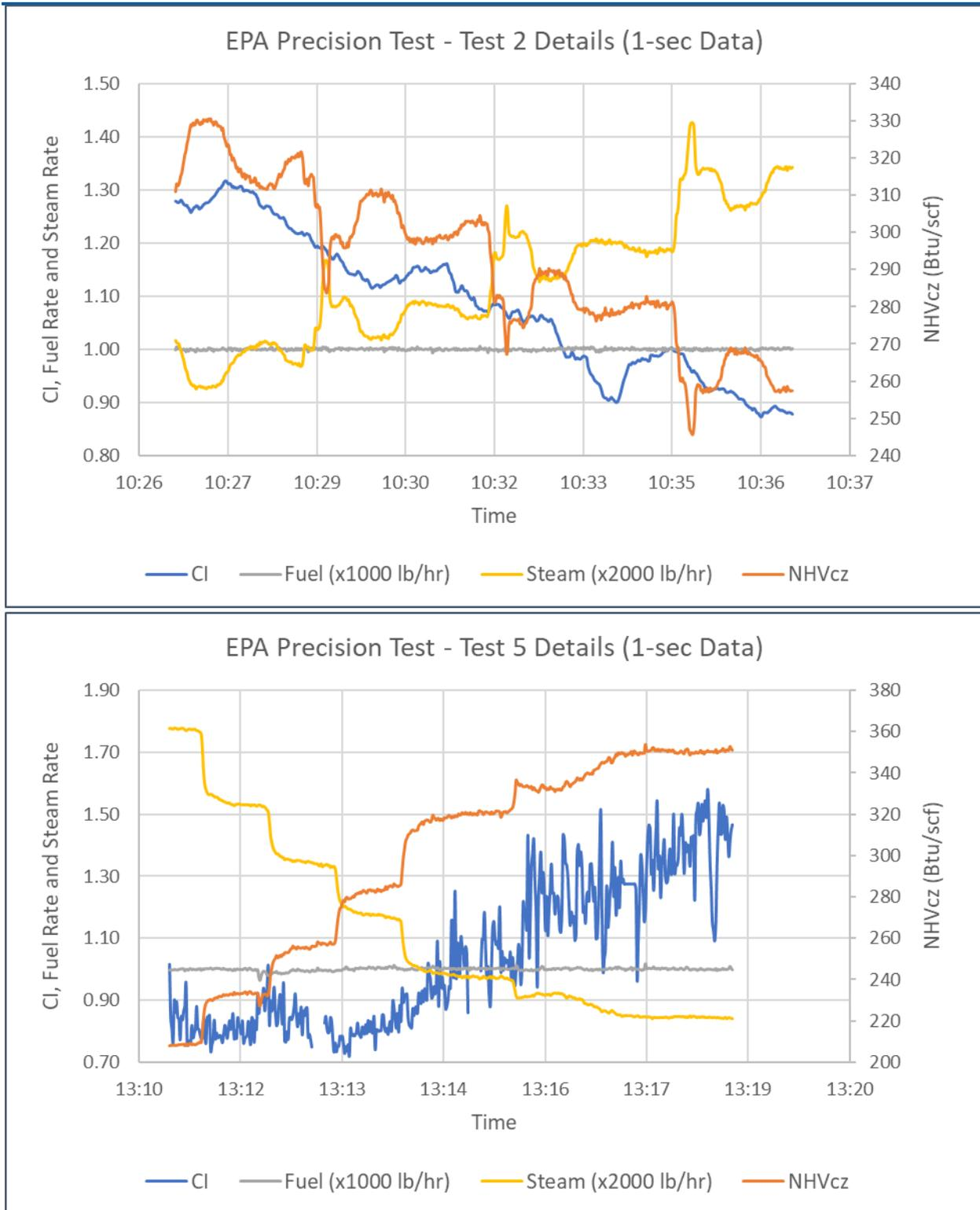
**Figure 5:** Time series plot at 1-second interval for CI, fuel rate, steam rate, and NHVcz for EPA Precision Test 2 (transition from high CE to low CE and Test 5 (transition from low CE to high CE).
