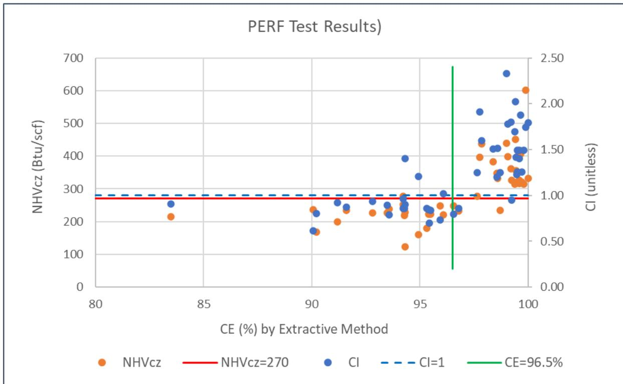
Figure 6: Comparison of the NHVcz method and the CI method based on the PERF flare study.
